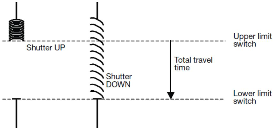
Note: The current position of the Blind during operation can also be determined with the help of the total move time. It is therefore important to measure and set the total move time as accurately as possible, particularly if the functions "Move to position" and "Status response" are used. Only then is it possible to calculate the current position of the Blind precisely.
