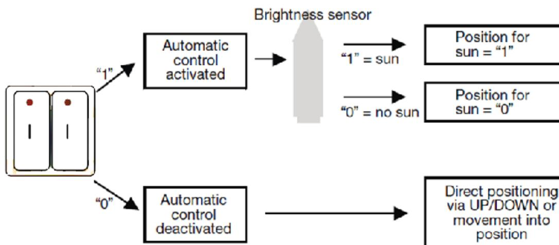
The Shutter actuator receives the information via the brightness sensor as to whether there is direct sunlight on the window. Once the delay period has elapsed, the Shutter actuator positions the shutter/blind according to the set Position for sun= “1” (sun) or Position for sun= “0” (no sun).
