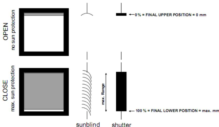
The functions described in chapters 5.3 for the “Venetian Blind” operating mode also apply to the “Shutter” operating mode (with the exception of the louvre adjustment function).
